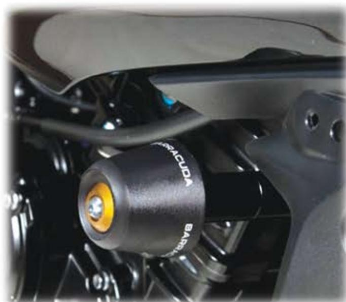
SEARCH AND FIND THE FIXING POINT ON THE MOTORBIKE BEFORE START TO MOUNTAIN, USE THE SPECIFIC THICKNESS AND BOLTS LIKE DESCRIBED IN THE PICTURE (SO YOU CAN GET THE RIGHT PROMINENCE FROM THE MOTORBIKE).
